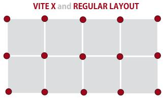
Cross section layout attained with the Cross VITE clips. Example of 12" x 12" tile using 140 clips for 100 sq.ft.
